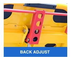
The back is controlled by a gas spring, and the back can be adjusted to the desired angle by just pressing lightly.
