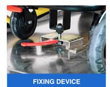
Each ambulance transporter comes with a fixing device that can be attached to the ambulance to prevent slipping.
