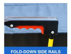
The foldable guardrail can prevent the patient from falling off the stretcher and causing secondary injury.
